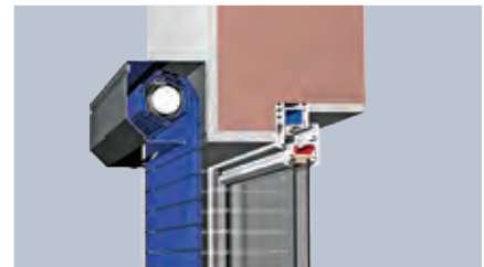
Facade installation (type C)
